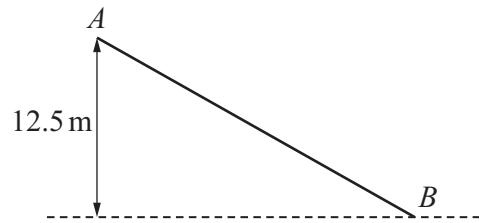
A particle of mass 7.5 kg, starting from rest at  $A$ , slides down an inclined plane  $AB$ . The point  $B$  is 12.5 metres vertically below the level of  $A$ , as shown in the diagram.
